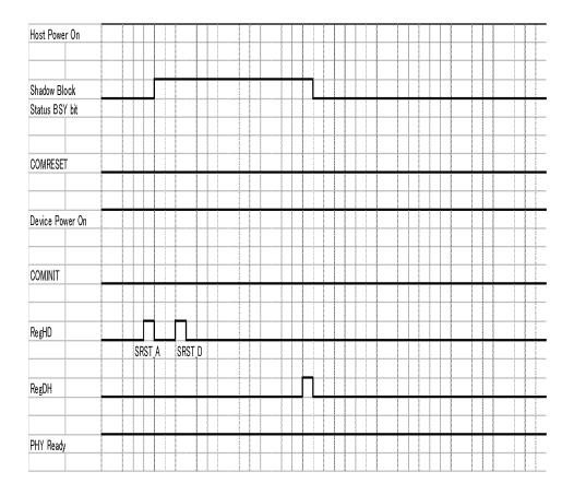
Figure 6.4 Response to a software reset
